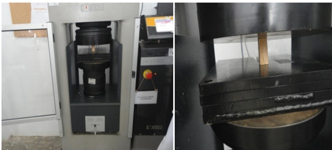
Figure 9: Essai de compression (Jdaidi, 2016)
